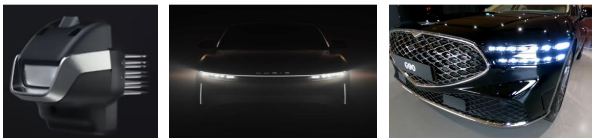
Figure 4. MLA head lamp module (left, Lucid), Lucid Air (middle) and Genesis G90 (right), first cars with MLA head lamp technology.
