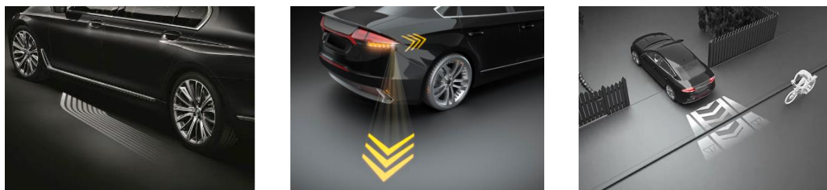
Figure 3. BMW welcome light carpet (left), new concepts for safety light carpets (middle, right).
